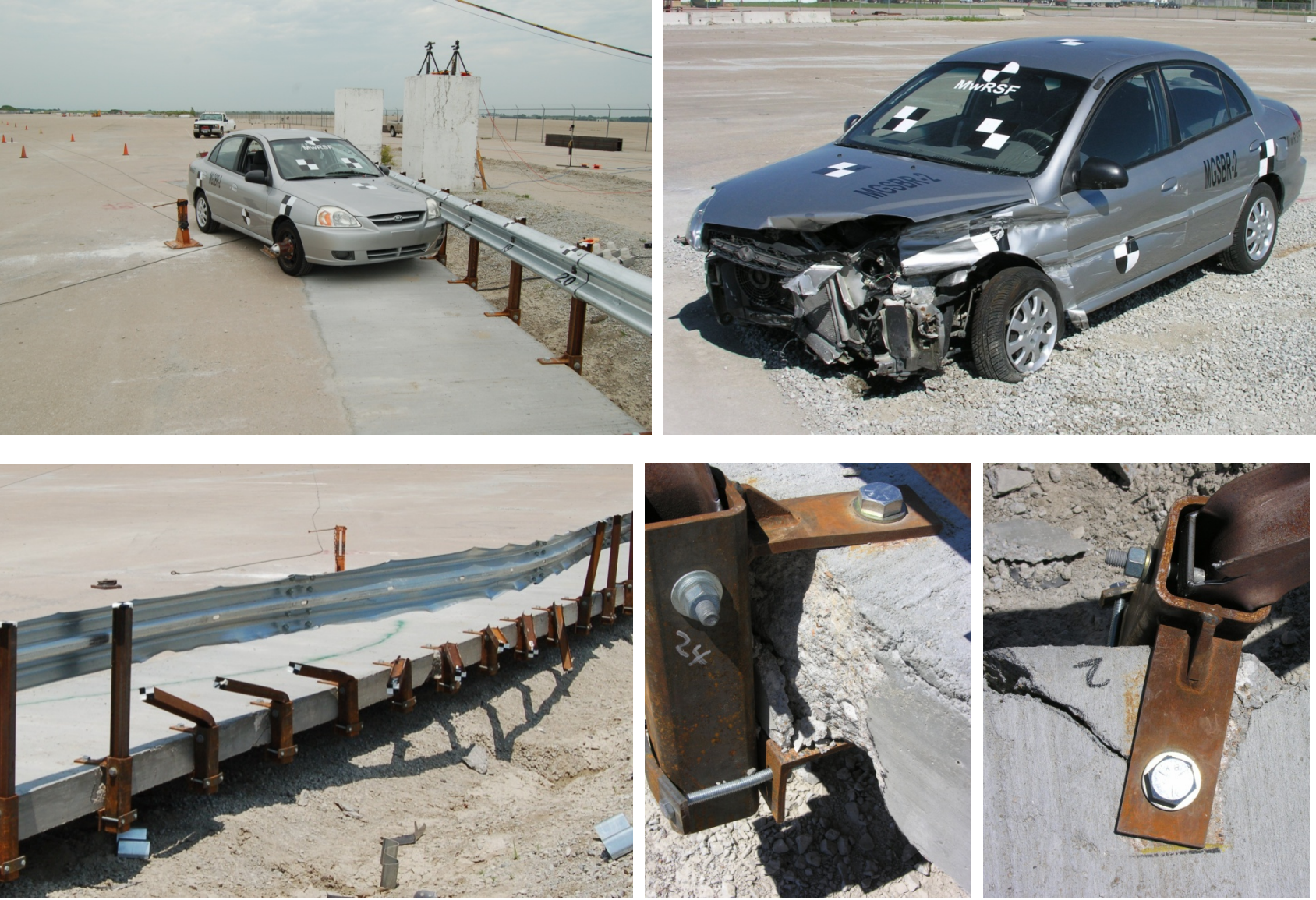
Figure 5. Impact Location, Vehicle Damage, and System Damage, Test No. MGSBR-2
